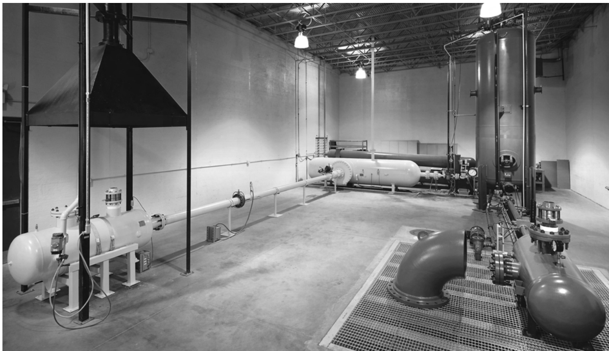
C.D.C. maintains an ASME accepted flow lab for conducting flow tests of rupture discs, pressure relief valves, and rupture disc / pressure relief valve combinations. Refer to bulletin 1-1106 for additional details regarding our flow test laboratory.
